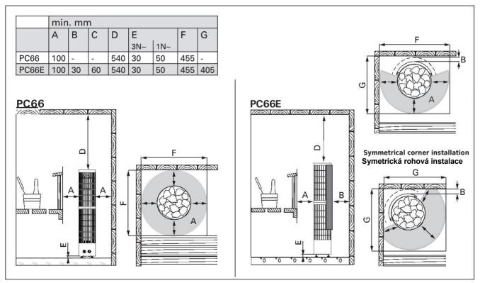
Figure 6. Safety distances (all dimensions in millimeters)
