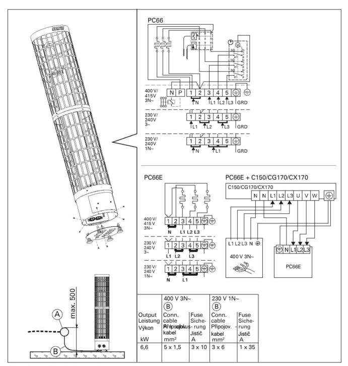
Figure 8. Electrical connections Obligations Elektrone subjections
