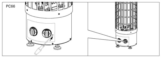
Figure 11. Reset button for overheat protector
